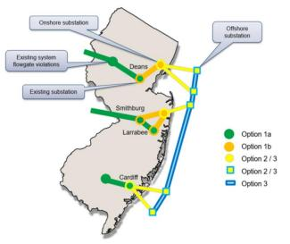
*Figure 4: Illustrative offshore wind transmission layouts.* <u>*Credit: PJM [7]*</u>
